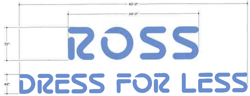
L.E.D. Internally Illuminated Channel Letter Set 511.00 SCALE: 3/16" = 1'-0"
